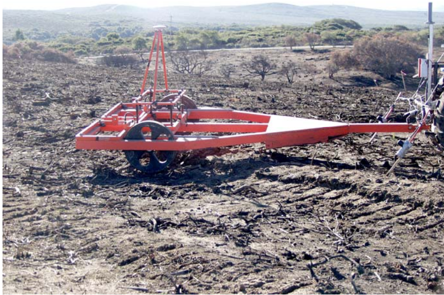
a. Towed-array with three EM-61 MKII sensors.
