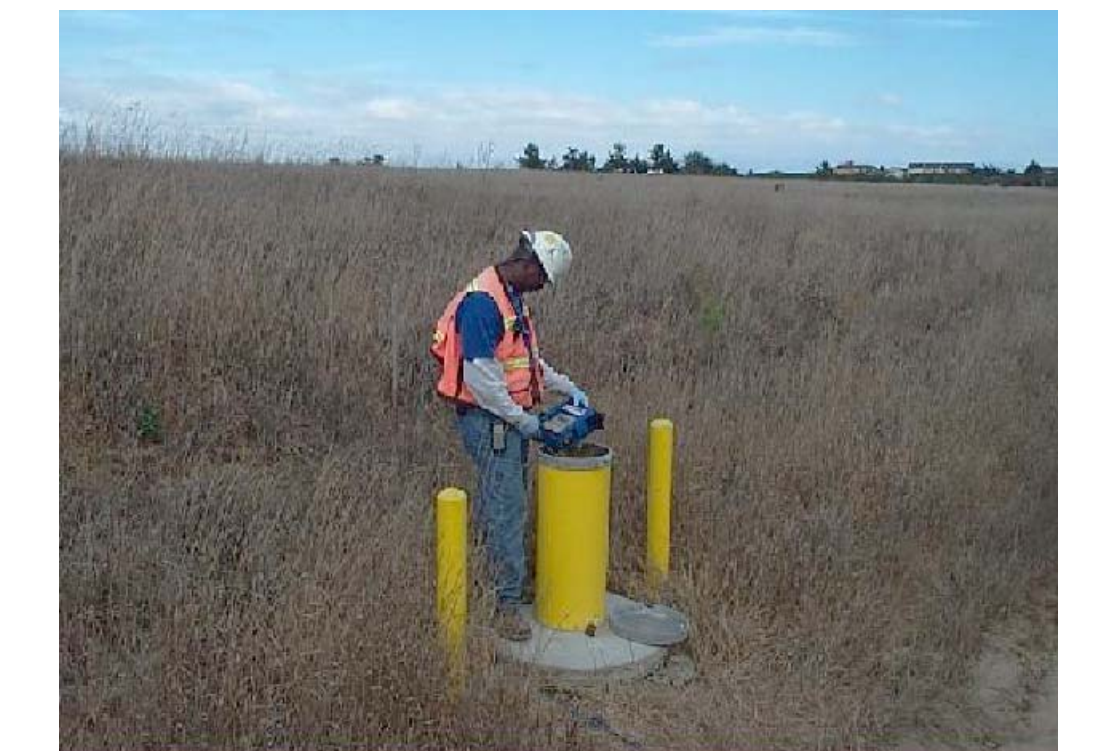
Landfill gas monitoring probes are monitored at least quarterly to ensure compliance with State regulations.
