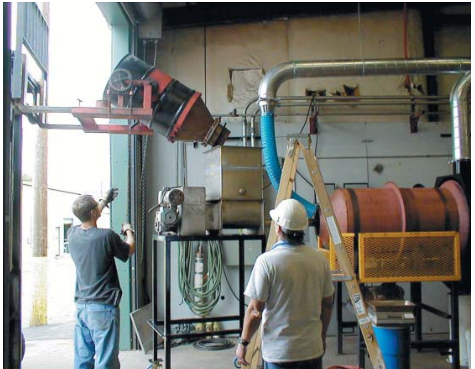
ITSI staff check a dry separation demonstration unit designed to remove bullets and bullet fragments from soil.
