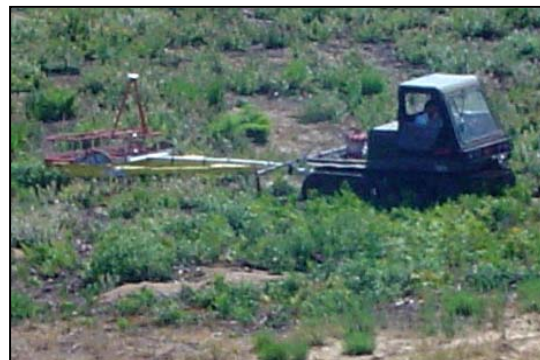
The EM61-MK2 towed array collecting geophysical data from MRS-Ranges 43–48.
