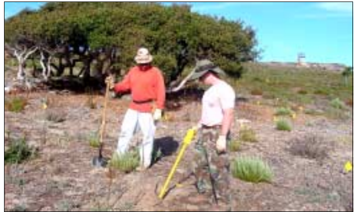
An instrument operator searches for OE with a magnetometer in OE-15SEA.1 as another team member prepares to dig any items detected
