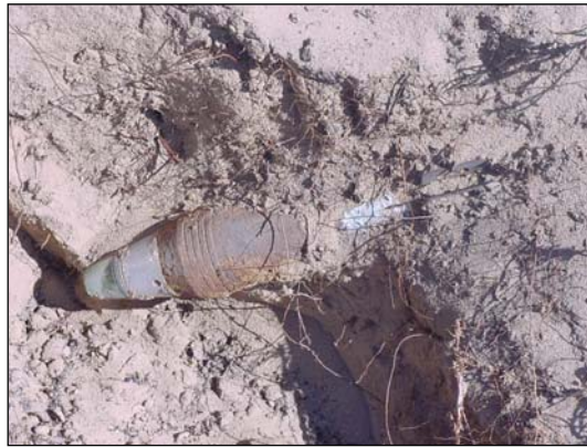
This 60mm high explosive projectile is one of over 8,000 MEC found so far in Ranges 43–48.
