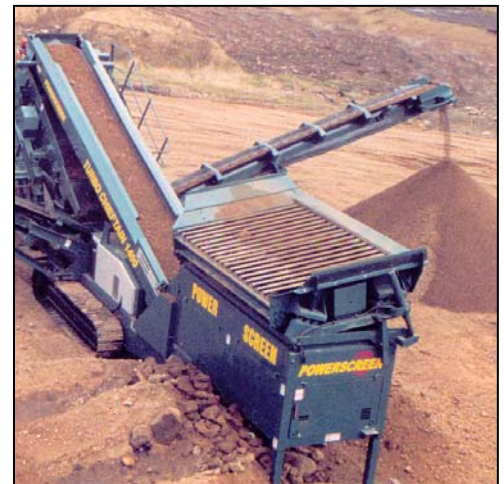
A sifter will be used to remove metallic debris from the top 2 feet of soil in the Range 45 area.
