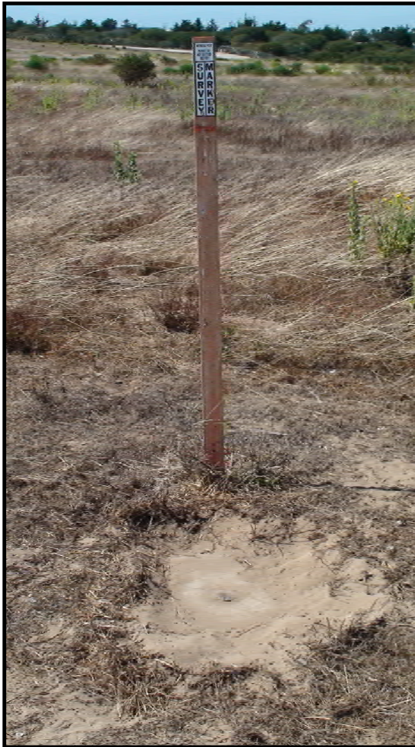
72. Area F Settlement Monitoring Plate SM-F1 (August 3, 2020)
