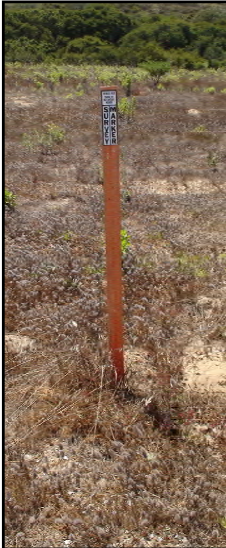
64. Area C Settlement Monitoring Plate SM-C1 (August 3, 2020)
