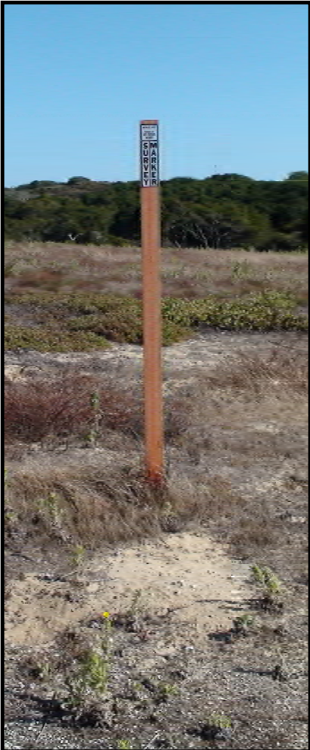
63. Area B Settlement Monitoring Plate SM-B1 (August 3, 2020)
