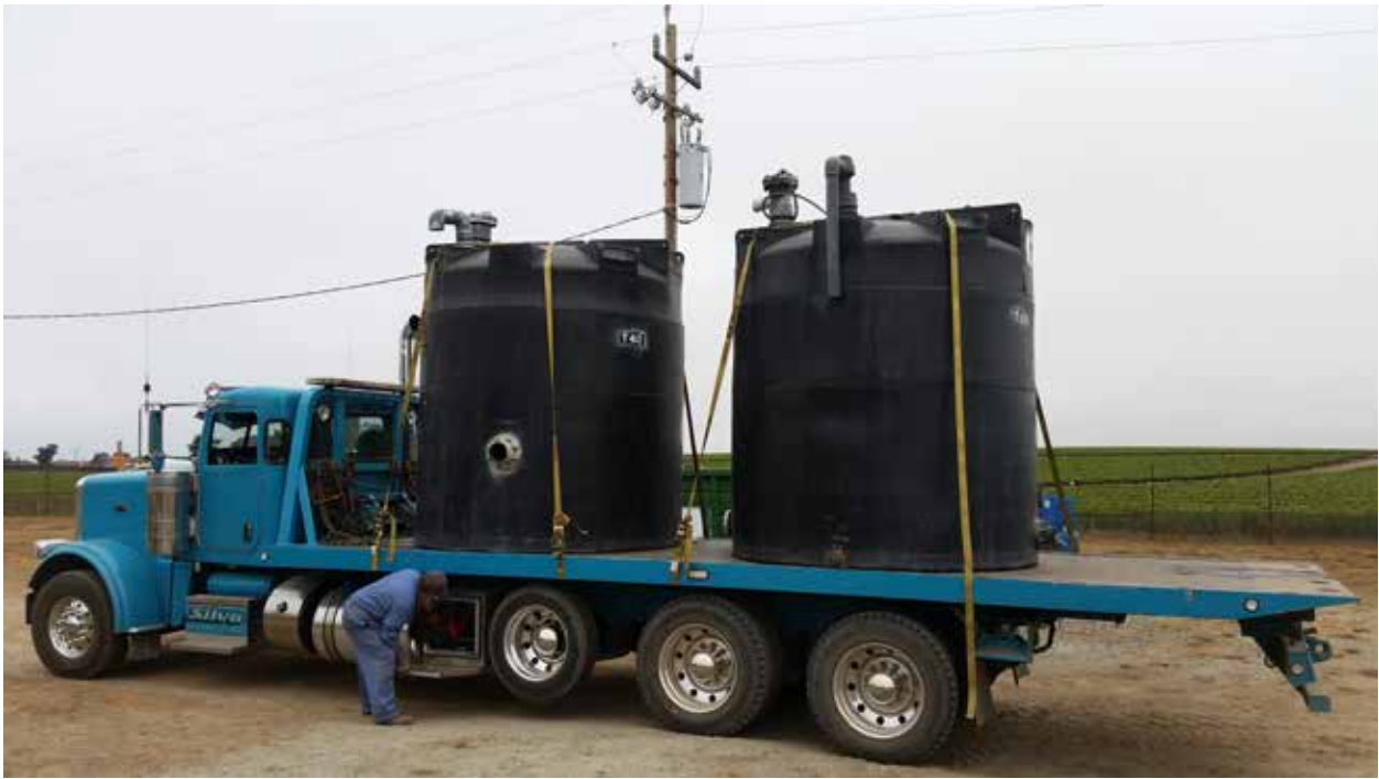
Influent and treated water holding tanks being loaded for transport
