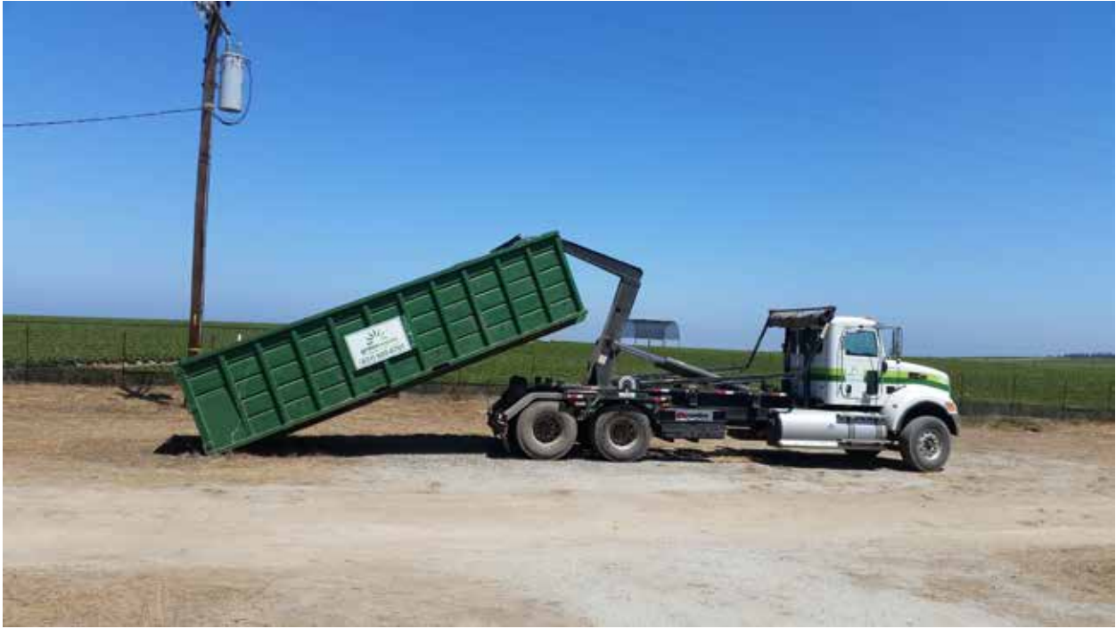
Loading roll-off bin at staging area for transport to disposal facility
