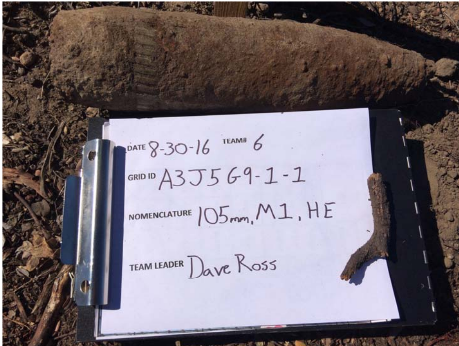
Photograph 7 – M1 High Explosive 105mm Projectile
