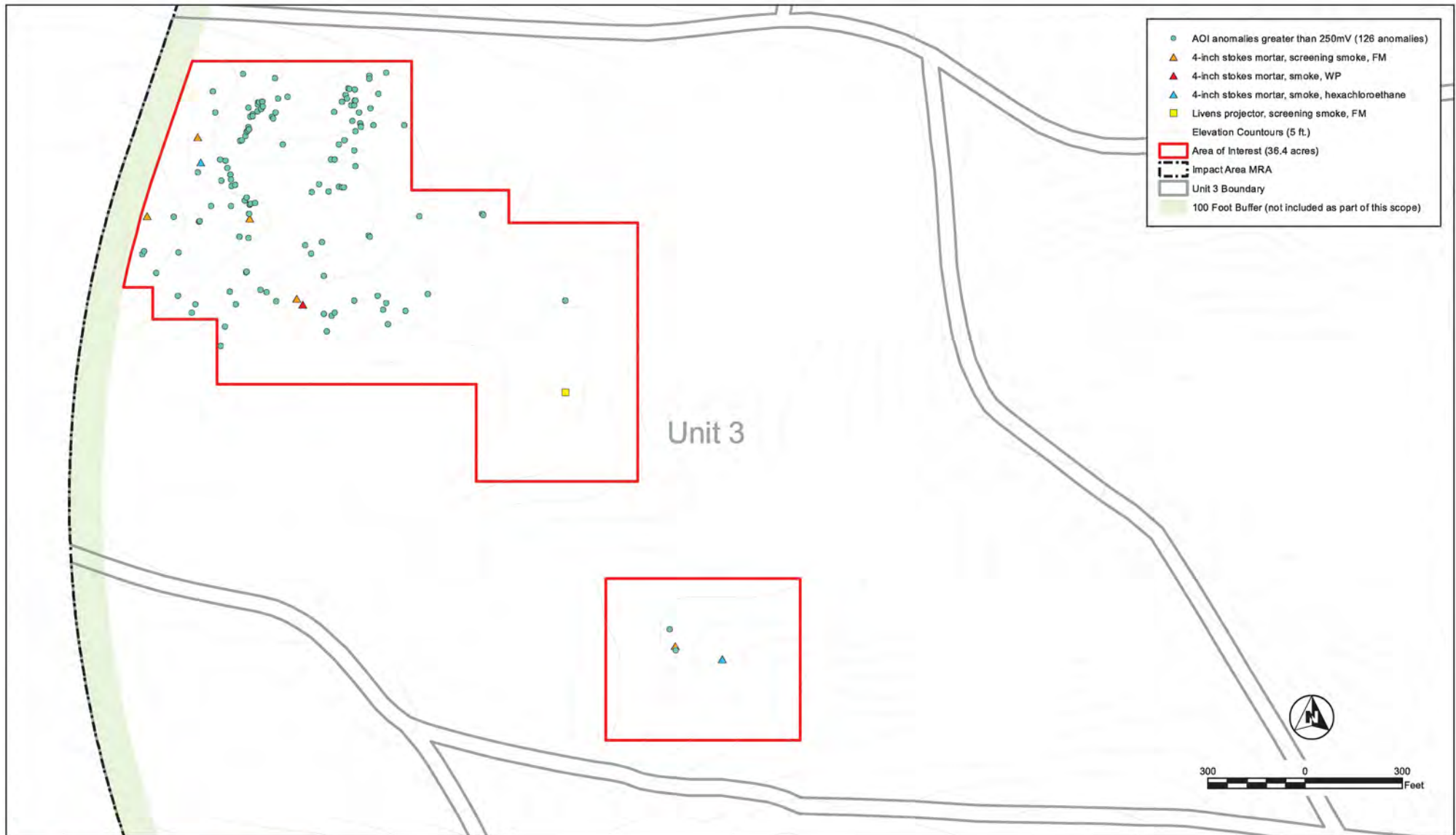
Figure 1 Unit 3 Area of Interest Stokes Mortar and Livens Projector Anomalies (to 12 inches bgs)
