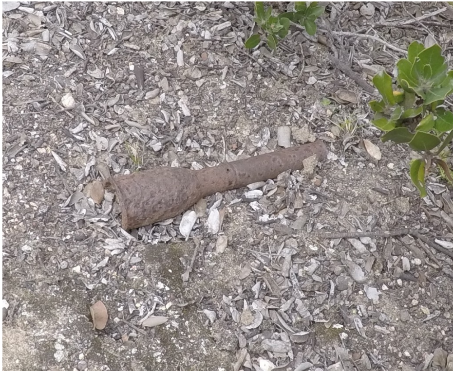
Photo 1B: Grenade, rifle, practice, M11 (MD). Located south/adjacent to Range 34 remediation area.
