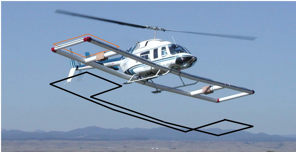
Figure 1.6: ORAGS-TEM system in flight. The red square line shows the large receiver coil position, and the black line represents the rectangular two-lobed transmitter coil layout.
