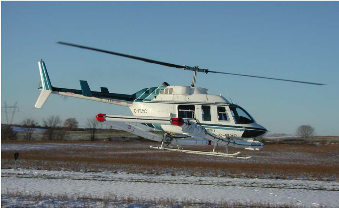
Figure 1.5: ORAGS-TEM airborne electromagnetic induction system similar to that used at Fort Ord.
