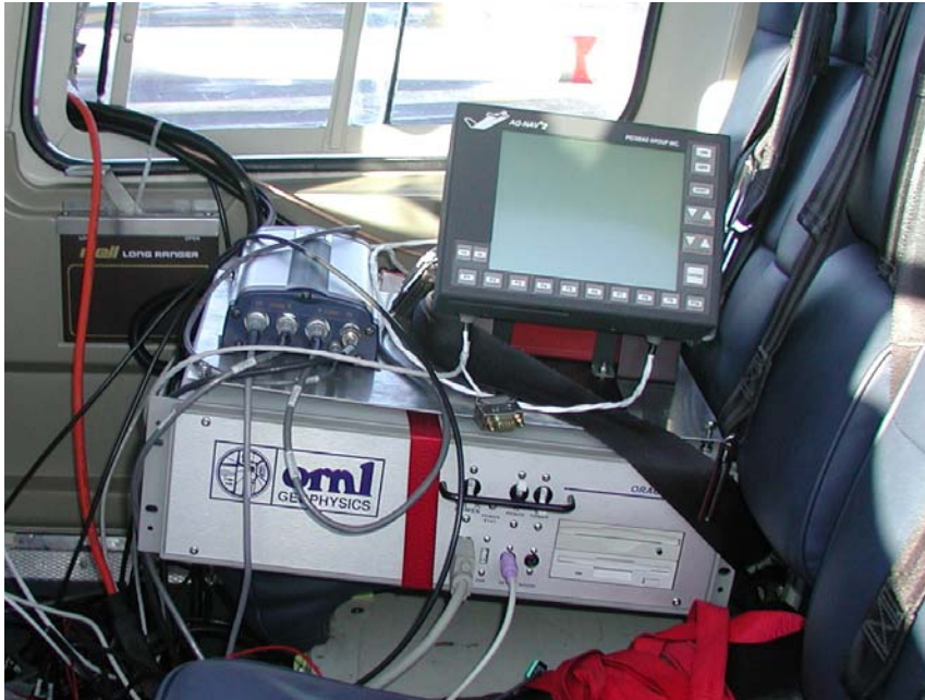
Figure 1.4: ORAGS-Arrowhead console as installed in the Bell B206L helicopter.
