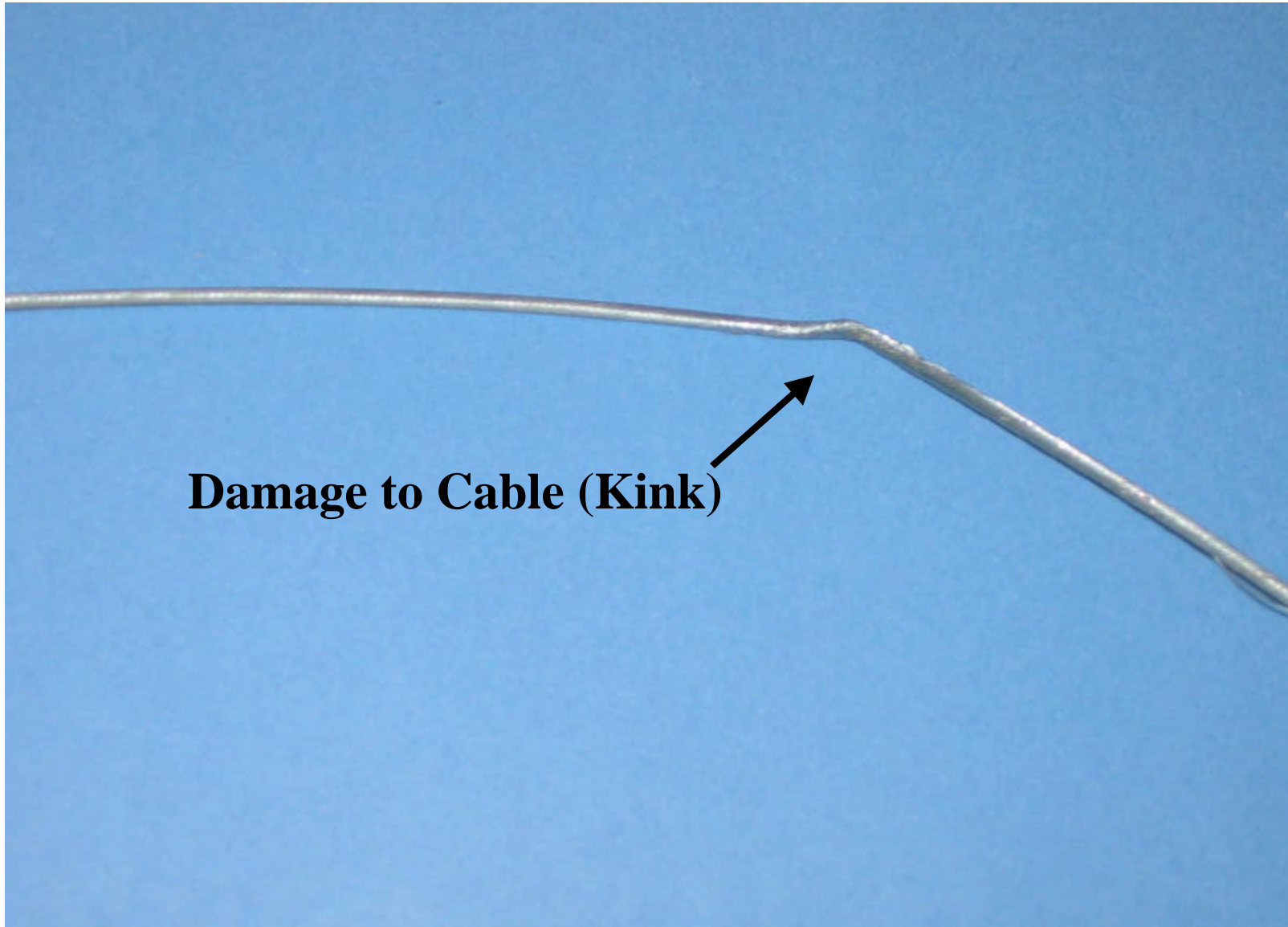
Pic.1 Identification of Cable Damage
