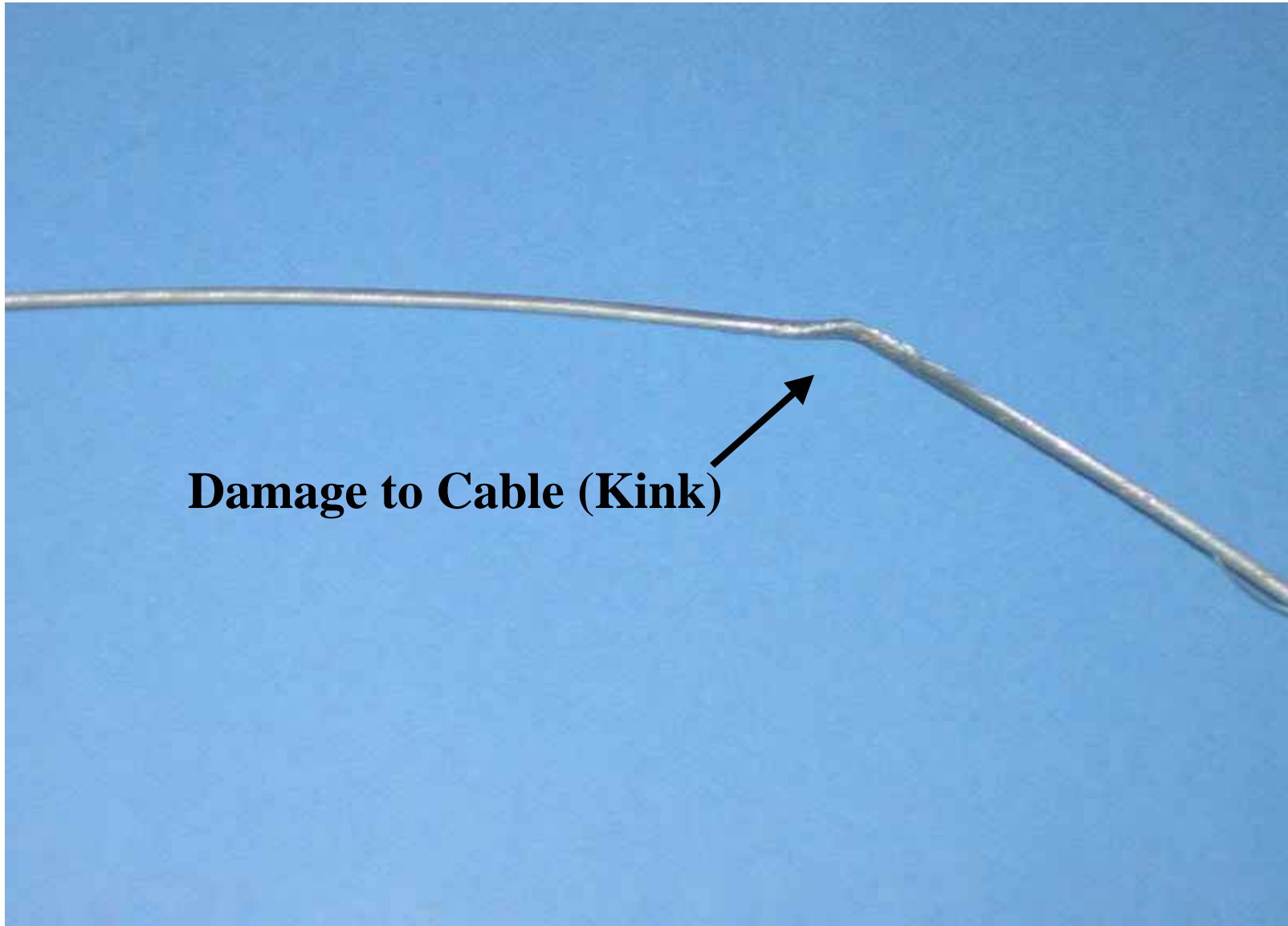
Pic.1 Identification of Cable Damage
