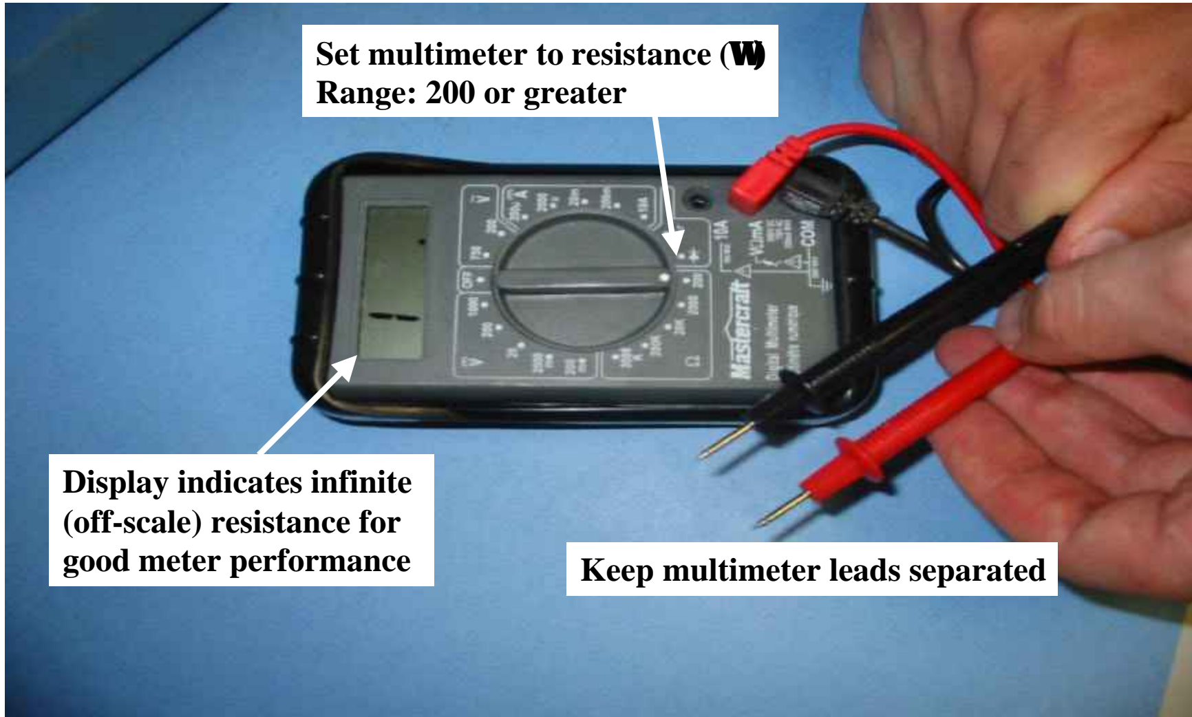
Pic.7 Test multimeter “open” resistance
